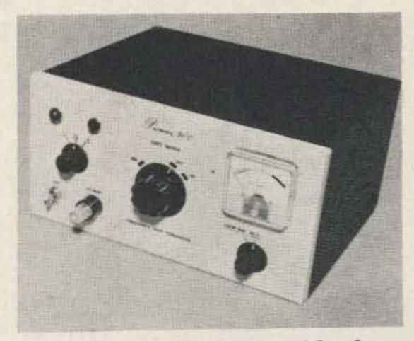
The Pioneer 900 is a tunable frequency shift converter which will accommodate any shift from 100 to 900 Hz. It has continuous tuning of shift range, permitting reception of stations using non-standard shift. The unit is completely solid state with 20 semiconductors and one integrated circuit. This
