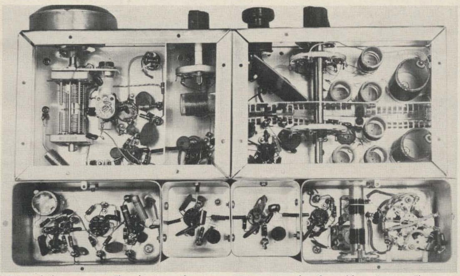
Wiring of the converter. The chassis in the upper right contains the rf amplifier circuitry. The upper lefthand chassis contains the vfo and 3.5-4.0 MHz output stage. The four small chassis on the bottom are, from the left, I MHz crystal-controlled reference and harmonic generator, two amplifier stages and the 1.75 MHz frequency discriminator.
