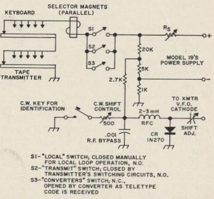
Fig. 5. The "Mainliner" frequency-shift keying circuit described by K8DKC in the May 1965 issue of QST. The resistor R<sub>s</sub> is adjusted for 60 mA through the selector magnets.
