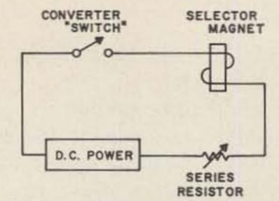
Fig. 4. Installation of the RTTY converter in the local loop to energize the printer from received RTTY signals.
