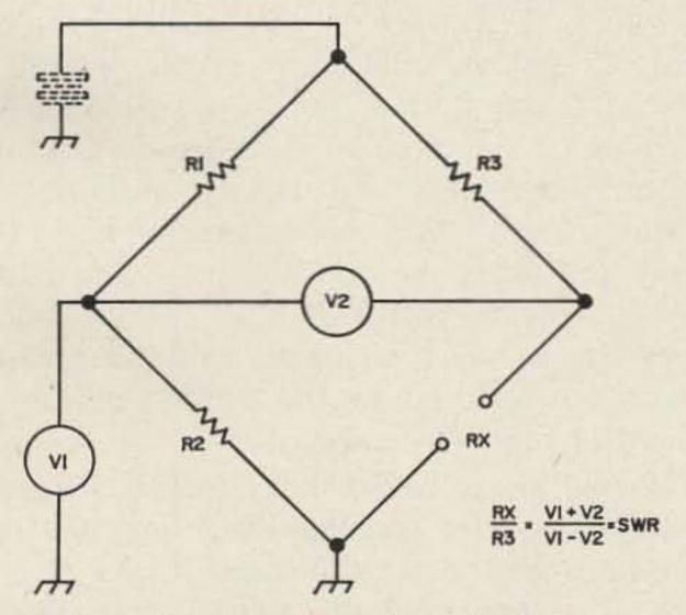
Fig. 2. Simplified diagram of SWR Bridge.  $V_1$  represents incident voltage and  $V_2$  the reflected voltage.
