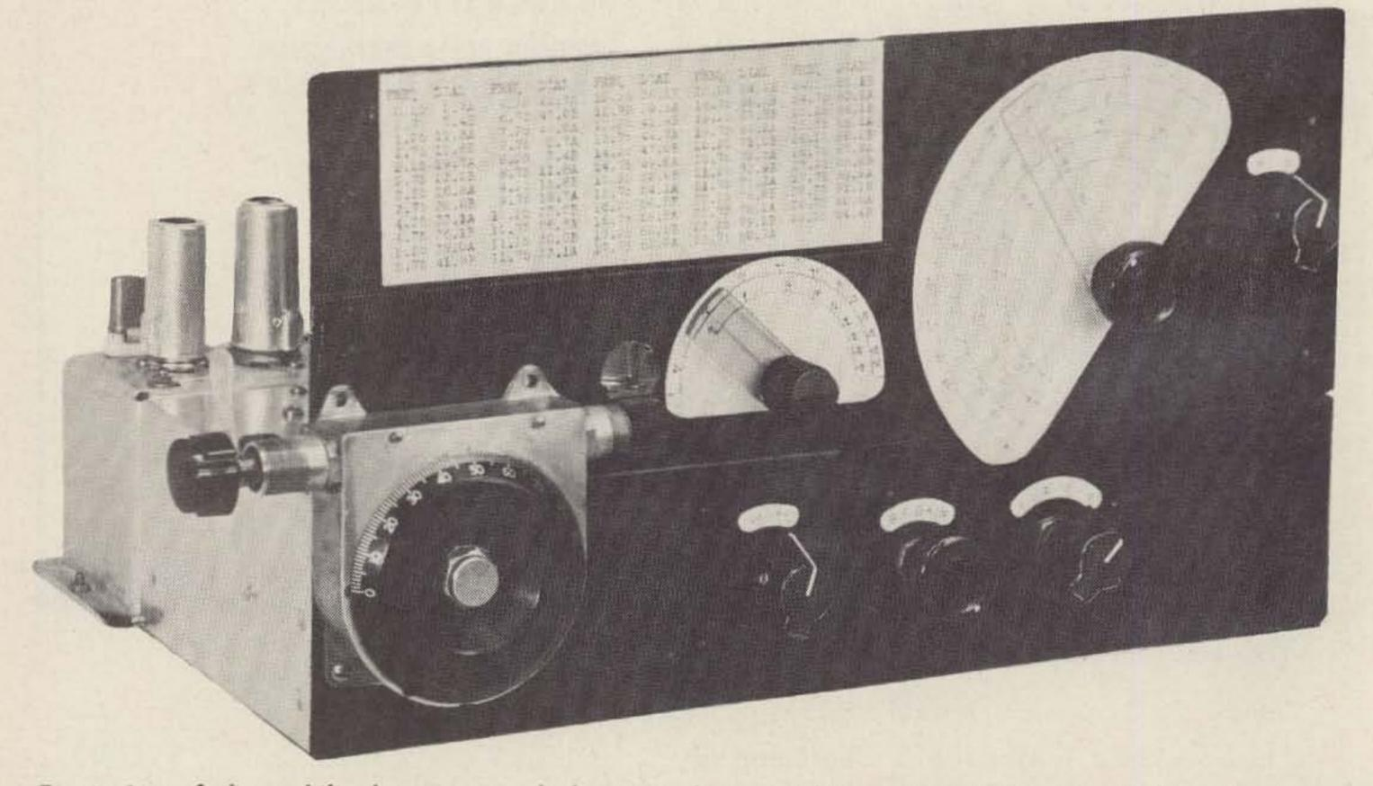
Front view of the stabilized converter which covers from 500 kHz to 29.75 MHz. The dial on the left is the tuning dial, the one in the middle is set according to the chart and the dial on the far right is the preselector.
