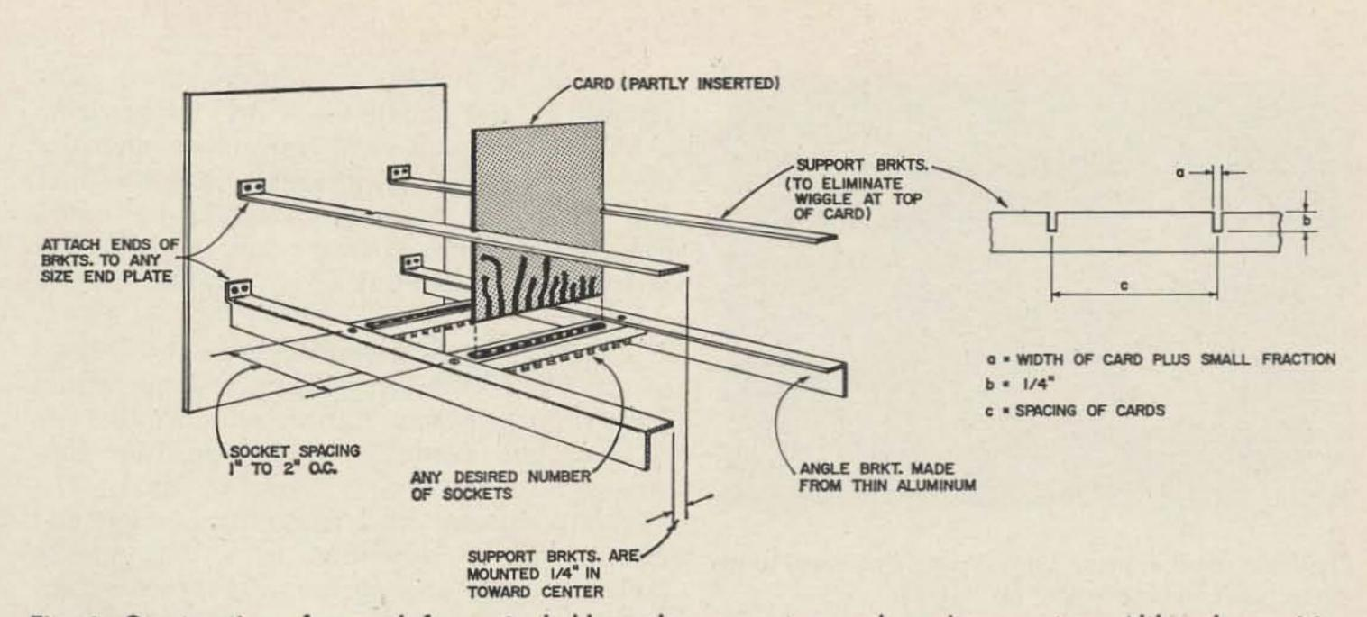
Fig. 1. Construction of a card frame to hold surplus computer cards and connectors. Although provision for only two cards is shown in this drawing, almost any practical number of cards may be held in one frame.
