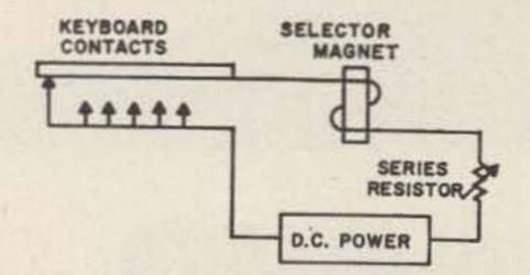
Fig. I. With the local loop shown here, the teletype operator can type on the keyboard and activate the printer for printing.
