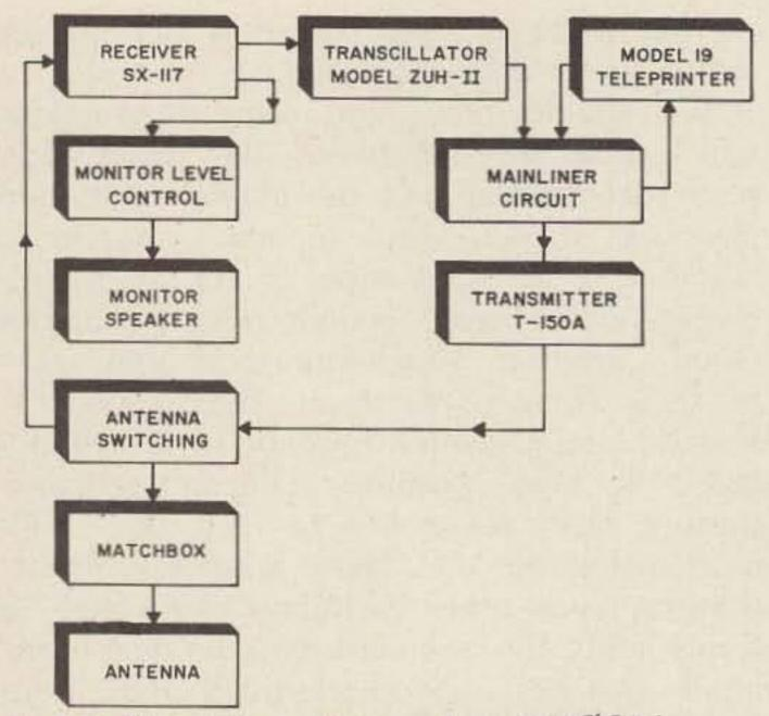
Fig. 6. The station setup used at WAØOBJ.
