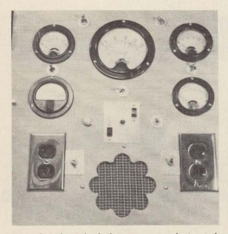
Note that the individual input receptacle to each of the four ammeters is not shown on the photograph. The reason for this is that I did not recognize the desirability of this feature until after the photograph was taken. All 'on'—'off' switches are turned 'on' by pushing the switches 'up'. All meter selector switches position by actuating toward the desired meter.
