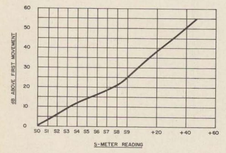
Fig. 1. S-meter calibration for SB-300. The unmodified curve is satisfactory. Without agc on the rf tube, the curve is too flat. Adding the parallel 100ohm resistor produces a good calibration, even between the 20-db points above S-9. The bend in the curves around S-9 is due principally to the scale markings; a flatter curve can be produced by using wider spacing on the graph.
