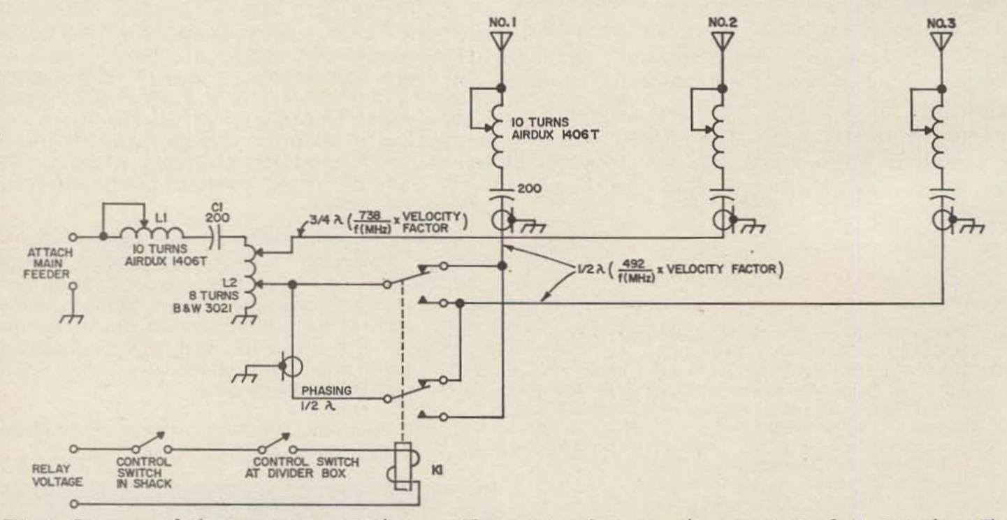
Fig. 1. Diagram of the 40-meter vertical array. The spacing between elements is 34 feet, 3 inches. The 1/2-wave phasing line using RG-8/U coax is 45 feet long (54 feet, 7 inches for foam coax). The 3/4 wave phasing line is 67 feet, 6 inches long (81 feet, 9 inches for foam).
