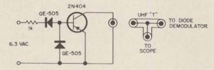
Fig. 1. Schematic of the solid-state chopper.
