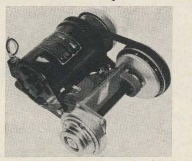
A portable alternator capable of delivering a constant power output of 2500 watts @ 115 volts, with a frequency variation of only  $\pm 2.5$  Hz has been announced by Prosser Industries, Inc. The model 2511A features an automatic transmission which compensates for input speed changes through 1800-3600 rpm to maintain a constant output of
