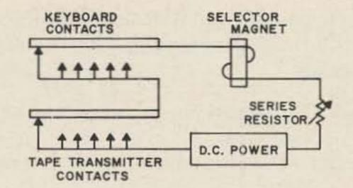
Fig. 2. With this local loop arrangement, the printer will print from either the keyboard or the tape reader.
