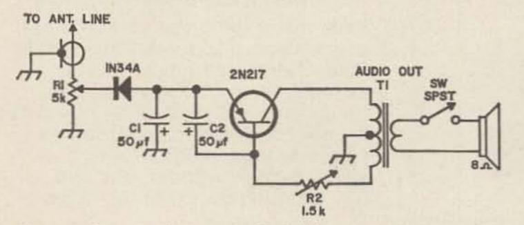
Fig. 1. Circuit diagram of the true parasitic monitor. The rf input is tapped directly onto the coaxial output connector of your SWR bridge. For power inputs over 250 watts, a small pickup probe may be used.
