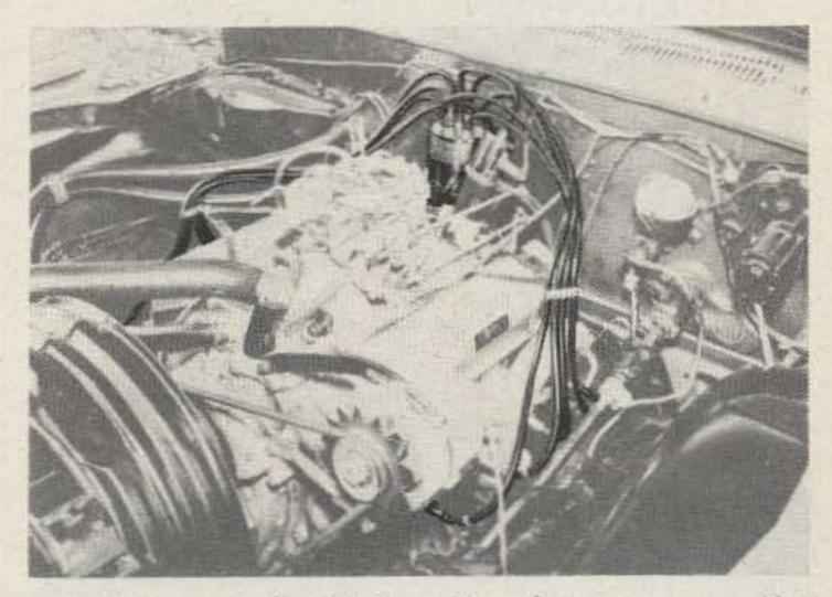
Installation of the Hallett Signal Saver on a V-8 engine (air cleaner removed).
