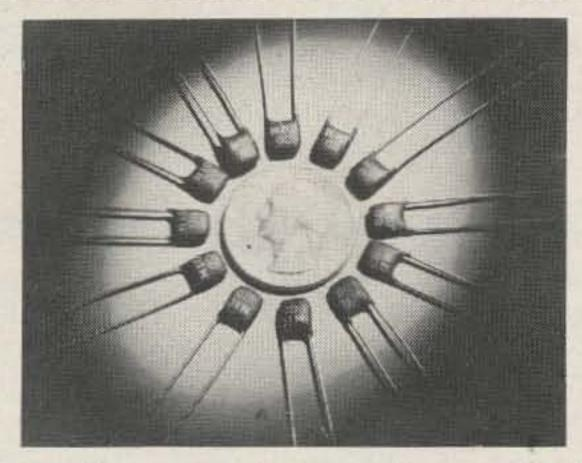
A smaller ceramic capacitor, with high stability, closer tolerance, and a higher capacitance per unit volume., than any previously designed is now available from Cornell-Dubilier Electronics.
