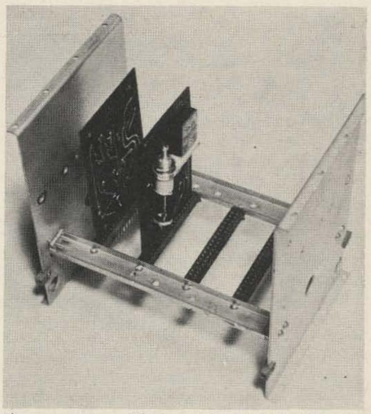
The computer card frame used by KIEUJ. If trouble is experienced with loose and wiggling cards, use the support brackets shown in Fig. 1.
