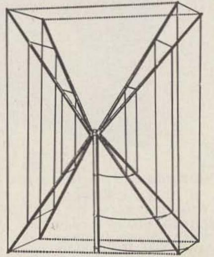
The Labgear 'QUAD' uses a spider construction providing optimum spacing on each band 10-15-20m. KITS AVAILABLE WITH OR WITHOUT BAMBOO ARMS.
