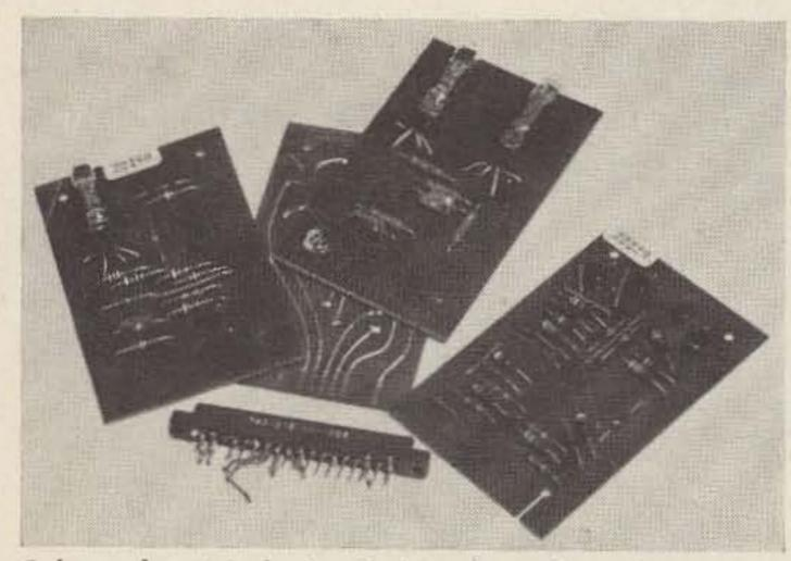
Salvaged printed circuit boards and socket.
