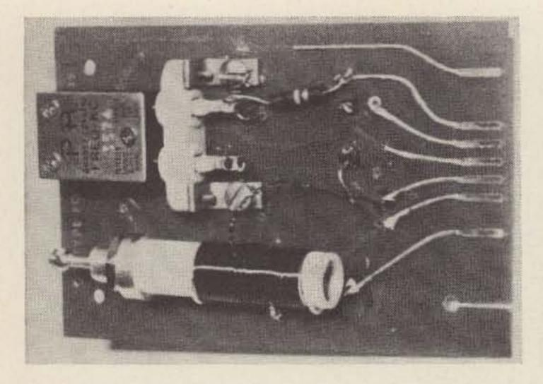
Oscillator card from a hybrid computer card transmitter under construction by KIEUJ.
