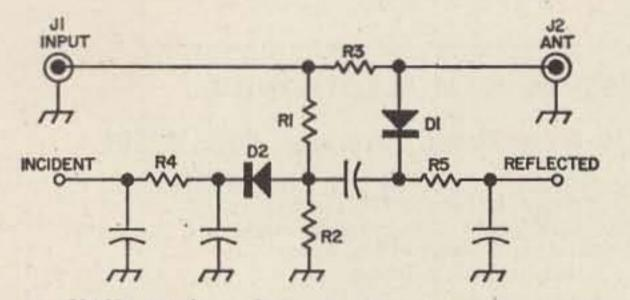
Fig. 1. SWR Bridge Circuit. See text for values of  $R_1$ ,  $R_2$  and  $R_3$ .  $R_4$  and  $R_5$  may be any matched value from 10 k to 47 k.  $D_1$  and  $D_2$  are IN34, IN54, or similar types. All capacitors are disc ceramic, .005 MF, 100V.
