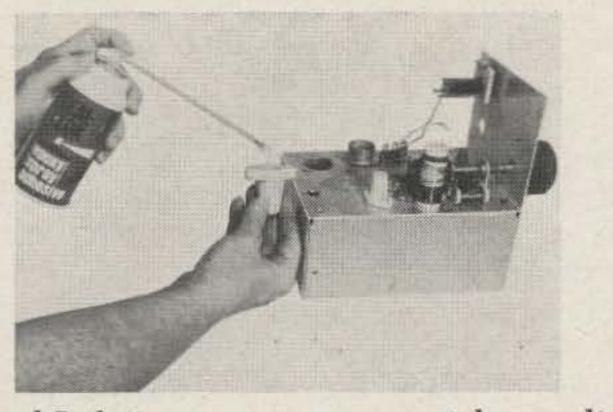
Leal-Lok is a one part material, supplied in 6-ounce aerosol cans, ready for immediate use. It is as easy to use as rubber cement and as strong as regular epoxy adhesives. It has a multitude of uses for such applications as fastening of brackets, handles, hardware, small parts and components as well as name plates and decorative accessories to panels, chassis, cabinets, and enclosures.
