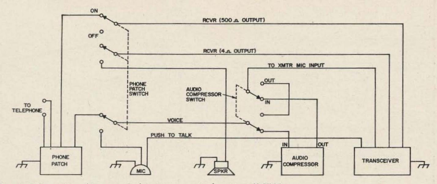
Fig. 1. Basic wiring diagram of the station control unit at K6ZHO.
