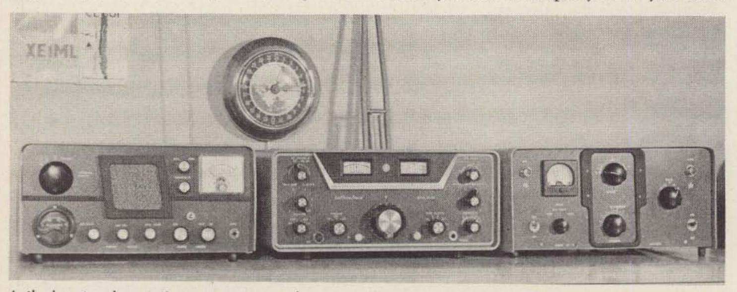
Author's setup has station acessory control unit on the left which matches SR-150 and homebrew copy of 30L-1 linear. Antenna switch is at top left and SWR meter is at top right. SR-150 plate meter is at lower left and lower knobs are for phone patch and audio compressor controls.
