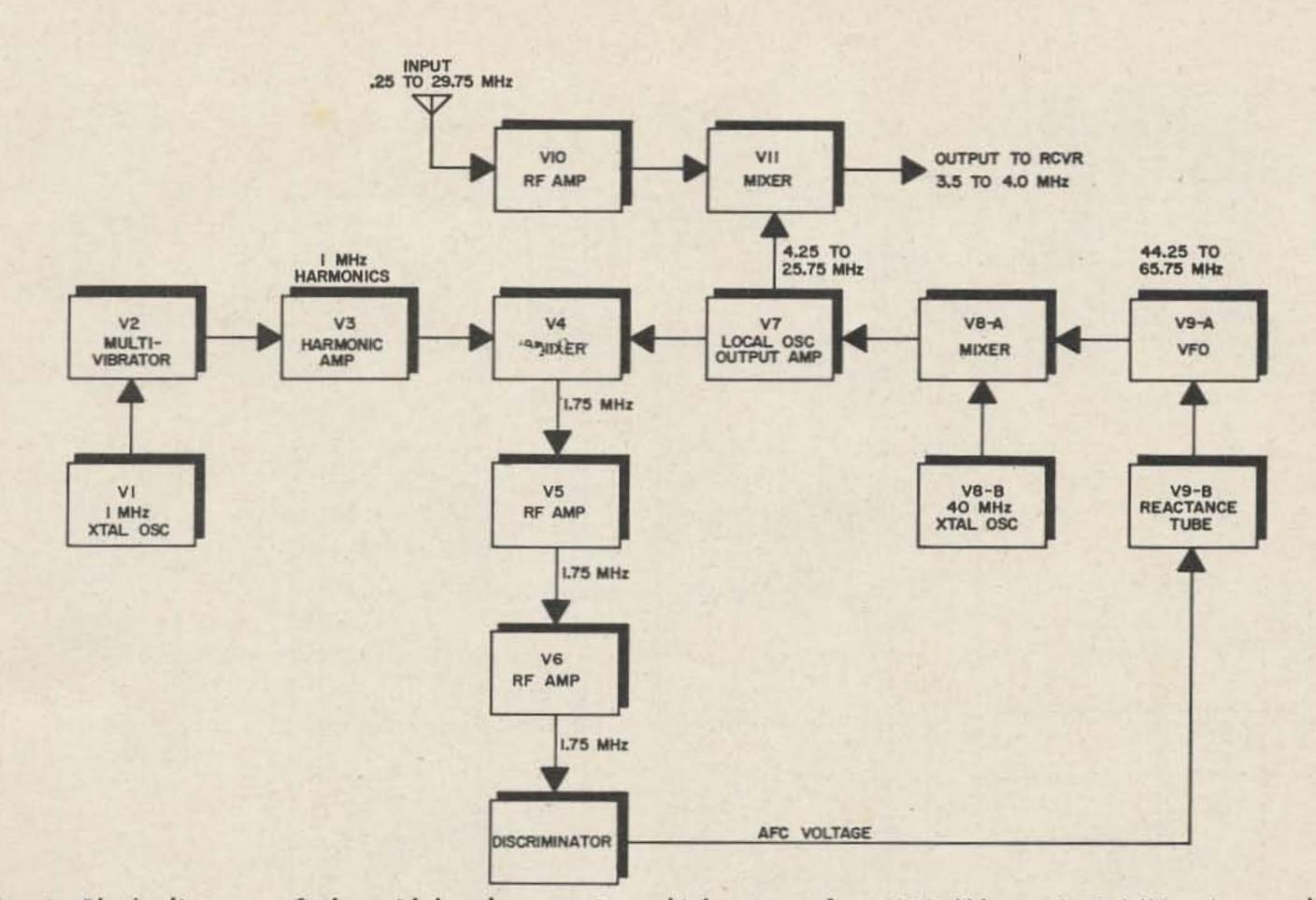
Fig. I. Block diagram of the wideband converter which covers from 500 kHz to 29.5 MHz. A complete description of its operation is given in the text.
