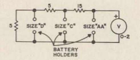
Fig. 2. Tester for dry cells. This tester puts a load on a standard carbon-zinc cell approximately equal to its 10-hour intermittent discharge rated load. A 40ohm load should be used when testing AAA or N size cells. A 9-volt transistor battery should be tested with a 250-ohm load and will give six times the voltage listed in Table 1.
