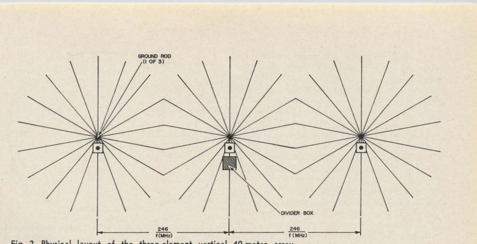
Fig. 2. Physical layout of the three-element vertical 40-meter array.
