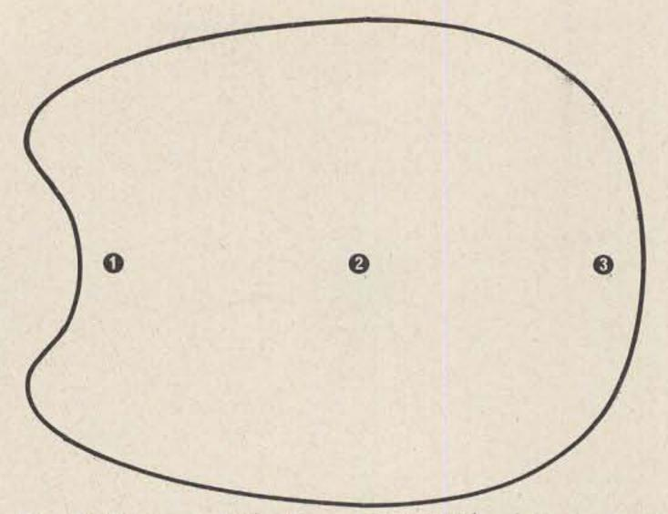
Fig. 3. Pattern of the array with 25% of the power at element I (0°); 50% of the power at element 2 at  $-90^{\circ}$ ; and 25% of the power at element 3 at  $-180^{\circ}$ .
