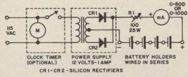
Fig. I. Typical dry cell charging circuit. See text for discussion of circuit values.
