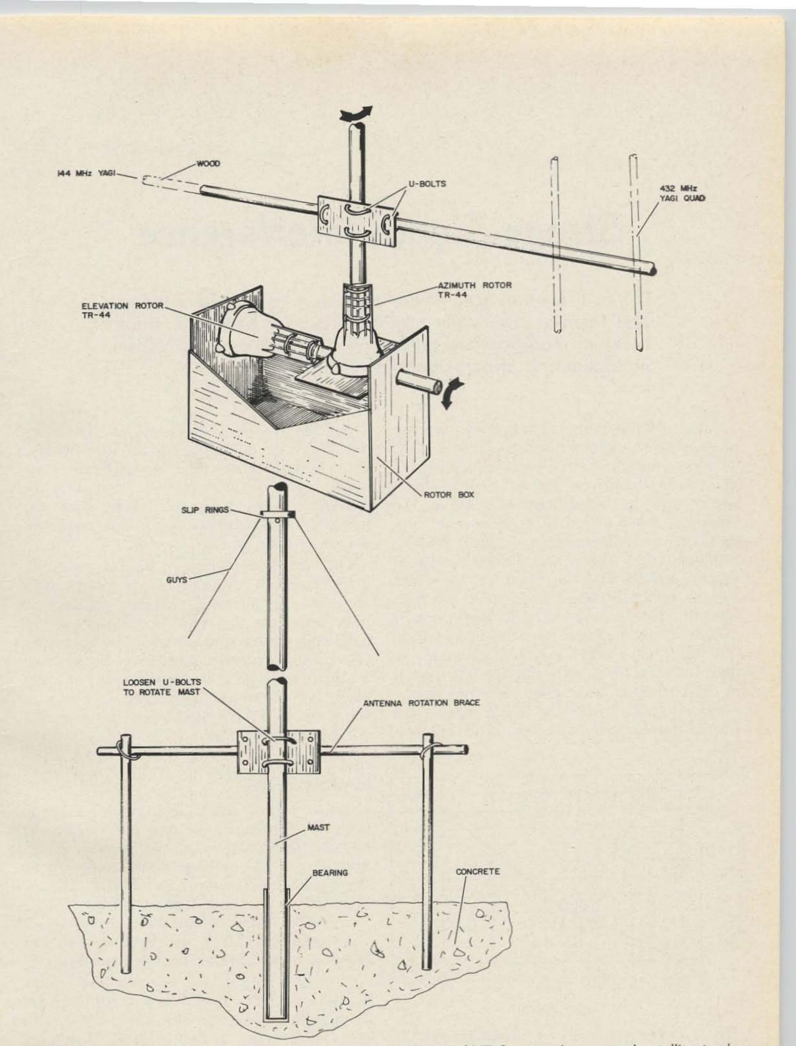
Fig. I. Construction of the simple antenna mount used by W4HJZ for moonbounce and satellite tracking.
